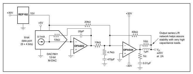
FIGURE 5. Digitally Programmable Power Supply.
