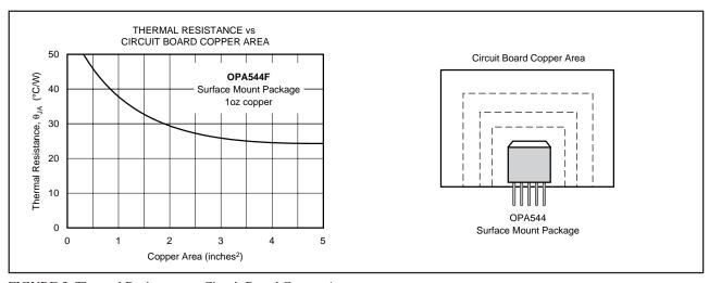
FIGURE 3. Thermal Resistance vs Circuit Board Copper Area.
