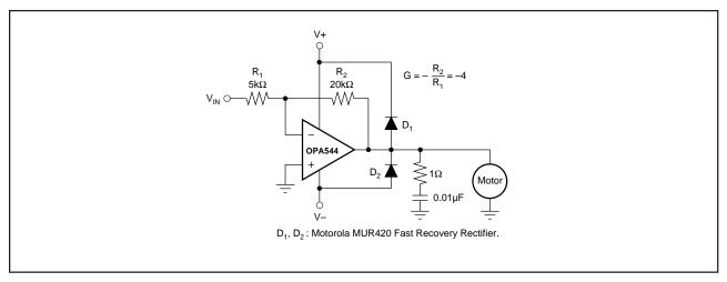
FIGURE 4. Motor Drive Circuit.
